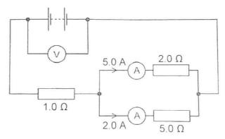
Determine the reading in the voltmeter.
