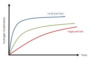
The frequency of effective collisions in Reaction 1 is higher than 2 because of the greater total surface area that is exposed for interaction between reactants.
