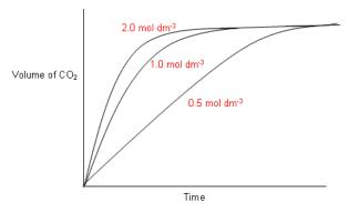
For the reaction with 2 moldm<sup>-3</sup>, the initial gradient of the graph is steeper compared to the rest, indicating a higher reaction rate.
