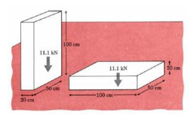
For a block with unique dimensions, the **smallest base area** gives the **greatest pressure**.
