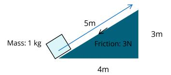
For the box to move up the slope, there is work done to overcome friction.
